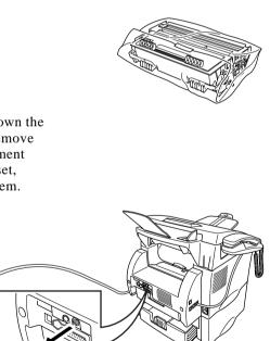
Carefully pick up the machine and remove Cassette #2 to pack it *separately*.
